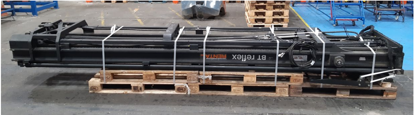
Fig 13 Mast securely banded to pallets
